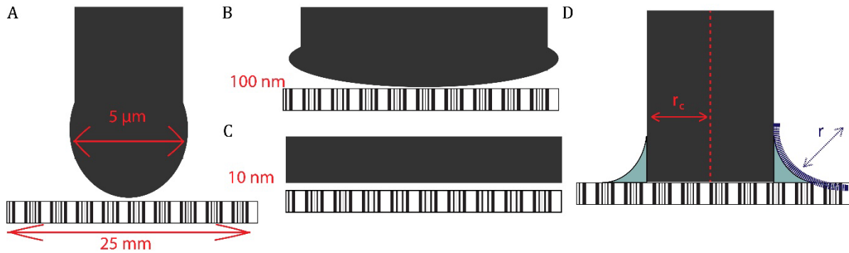
Figure 7-2: (A) General schematic of the AFM tip used in this study approaching a planar plastic surface (B) Zoomed into the nanometer scale, the micron sized spherical tip becomes more planar from the perspective of the plastic surface (C) Once you reach the 10 nm scale, the radius of the AFM tip used in this study, it is essentially a plane-to-plane interaction (D) Using a planar assumption due to the micron scale (relatively large) AFM tip used in this study, this interaction can be approximated by a standard flat cylinder tip-planar sample surface schematic where the meniscus force is a result of the blue shaded region (Farshchi-Tabrizia et al., 2008).
