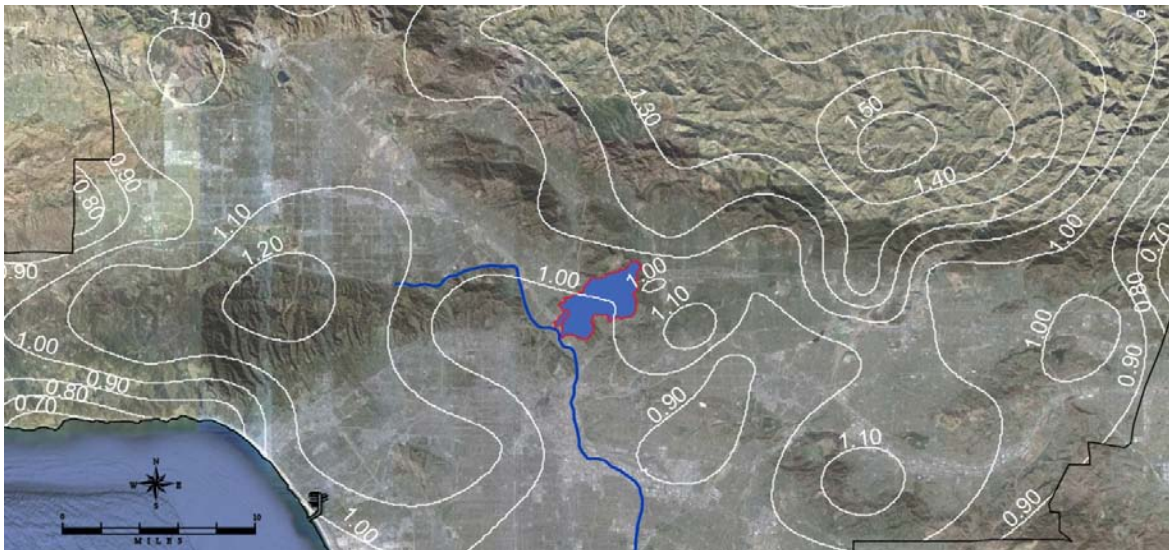
Figure 5: The 85 th percentile isohyets for Los Angeles County. Two sub-watersheds (shown in blue) fall around an average rainfall of 1.00" per 24 hours.
