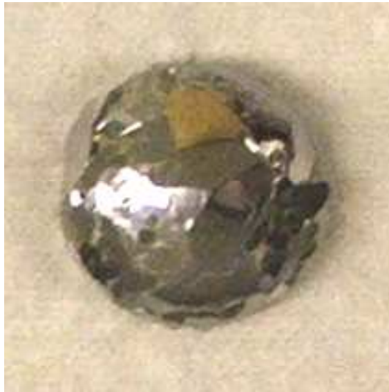
Figure II.1: Photograph of a polycrystalline sample of URu 1.65 Re 0.35 Si 2 , with a diameter of approximately 2 cm, formed in an arc furnace. The large facets on the surface that give the sample its disco ball appearance are oriented perpendicular to the [001] direction.
