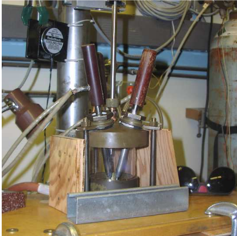
Figure II.2: Photograph of the tri-arc furnace used in the Czochralski growth of \text{URu}_{2-x}\text{Re}_x\text{Si}_2 single crystals. The pulling rod is inserted into the chamber through an o-ring assembly at the top. A motor rotates the rod while a separate drive translates the rod upward. During operation of the arcs, a UV filter is placed between the operator and the furnace.
