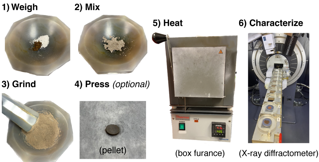
Figure 1.1: The basic procedure for solid-state synthesis. Note that Steps 2-4 are frequently included to increase the total interfacial contact area between differing precursor crystallites but are not explicitly required in all cases.
