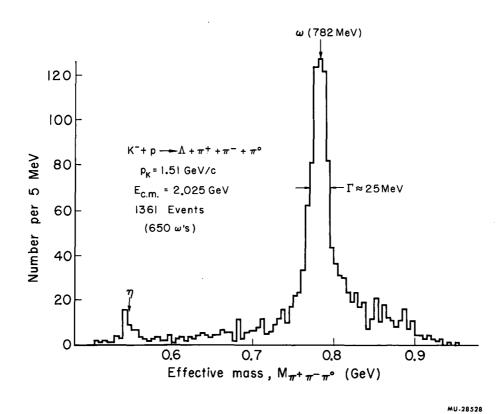
Fig. 1. Three-pion effective mass spectrum in the reaction  $K^- + p \rightarrow \Lambda + \pi^+ + \pi^- + \pi^0$  at 1.51 BeV/c. About 650  $\omega$ 's are seen above background. The width of the  $\omega$  peak is due chiefly to measurement error.
