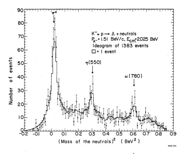
Fig. 3. Mass of missing neutrals in the reaction  $K^-+p\to\Lambda$  + neutrals at 1.51 BeV/c. About 40 neutral  $\omega$  decays (presumably  $\pi^0$  +  $\gamma)$  are seen above background.
