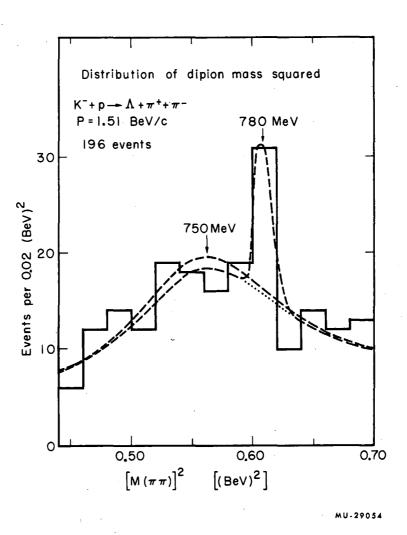
Fig. 8. A portion of the pion-pion mass spectrum shown in Fig. 7. One of the curves represents a fit to the data with a P-wave  $\rho$  meson and constant background; the other curve represents a fit with a P-wave  $\rho$  plus background and also a narrow Gaussian centered at 780 MeV to represent the  $\omega$  meson.
