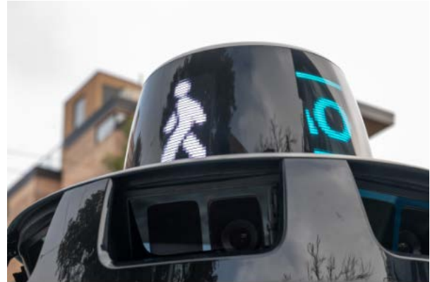
Figure 2: eHMI on an autonomous vehicle displaying a pedestrian walking sign. 25
