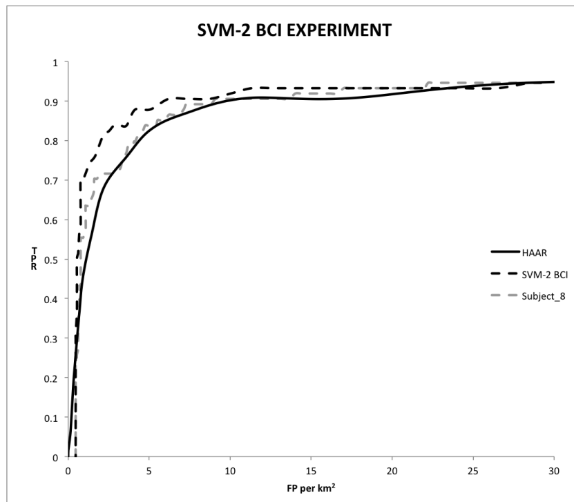
Figure 8.18. The vertical axis is true positive rate (TPR) and the horizontal axis is false positives per square kilometer (FP per km 2 ). This compares the receiver operating characteristic (ROC) curves of the three stage BCI experiment concluding with the SVM classifier, the Haar-like feature classifier, HAAR , and the two stage BCI using Subject 8, Subject_8 . For all curves, the Haar-like feature classifier portion uses a threshold of two.
