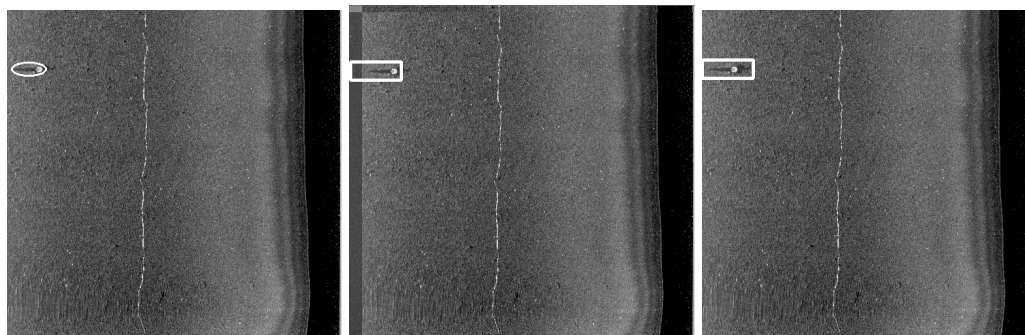
Figure 5.11. Example of a MLO along the image edge. The left image is the default search, which does not find the MLO and is shown by an ellipse. The padded image is shown in the middle, with the target detection shown by a rectangle. The right image shows the detection within the bounds of the original image via a rectangle.
