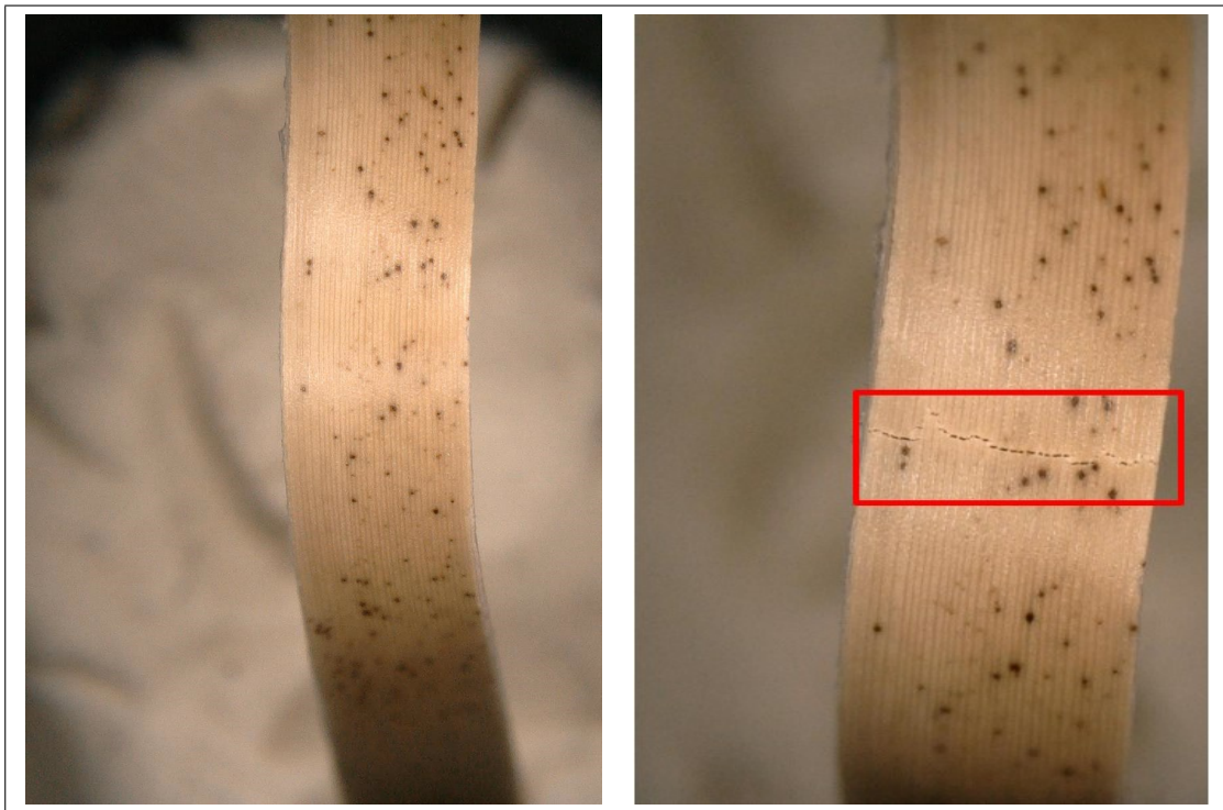
Figure A.37: 1yr Sample 4 Apex Before and After Compressive Testing.
