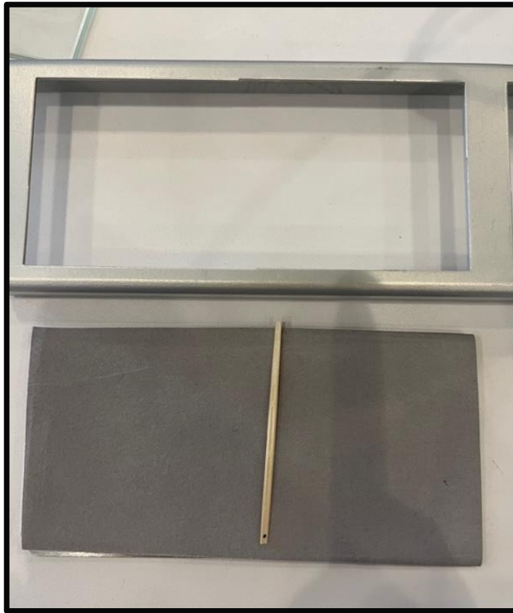
Figure 6. One sample from the 7-year age group was prepped for MFT testing with the gray background and the orientation of the sample in the tray.
