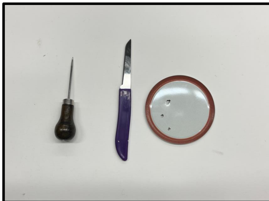
Figure 4. Tools used to prep the Sólýla samples. An awl, small knife, and a metal sizer.
