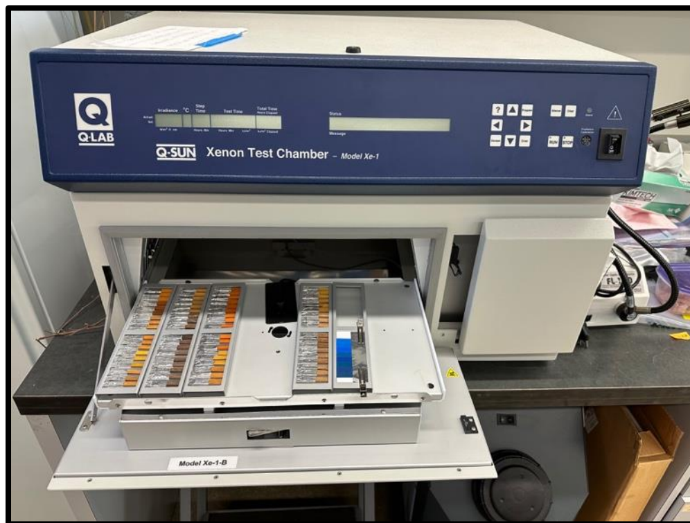
Figure 5. Q-Sun Xenon Test Chamber with Cheyenne Caraway's dyed rivercane samples. An example of how samples were wrapped and prepared with foil. Picture courtesy of Cheyenne Caraway
