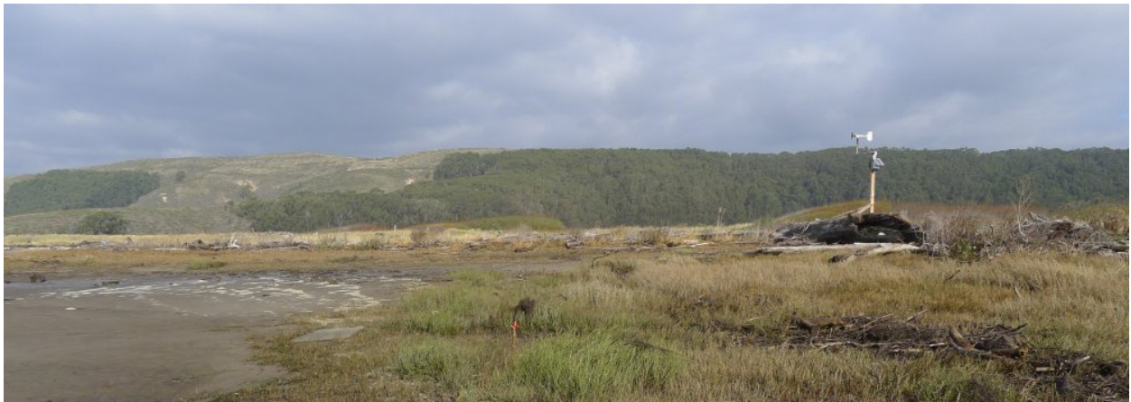
Figure 2.5: An anemometer made wind measurements approximately 3 m above the water level in the Pescadero estuary.
