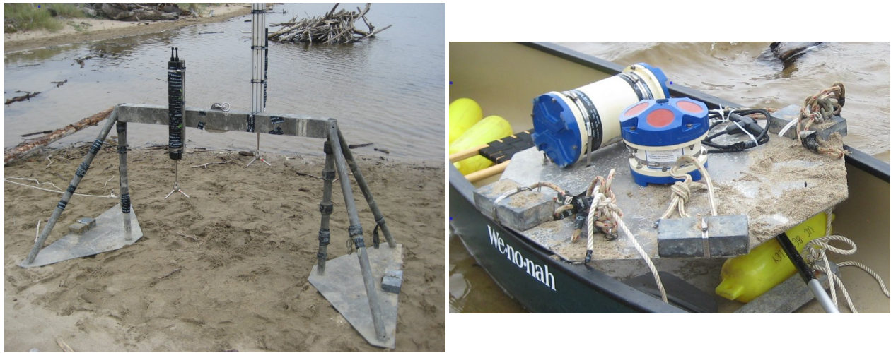
Figure 2.4: Photographs of downward facing ADVs and an upward facing ADCP used in field deployments.
