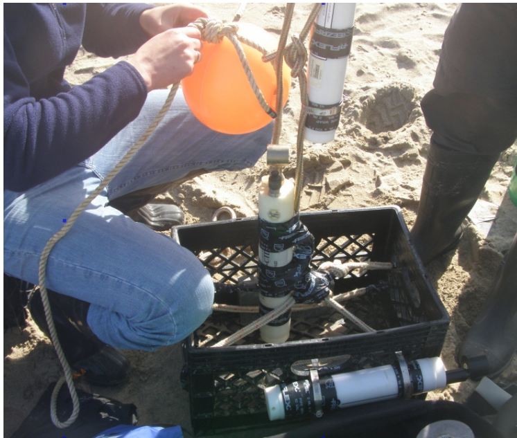
Figure 2.3: A mooring consisting of several CTDs and buoys attached to a weighted milk crate. Bed CTDs were attached 0.2 m above the bottom of the milk crate.
