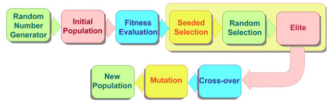
Fig. 17. Structure of genetic algorithms and genetically based operators.
