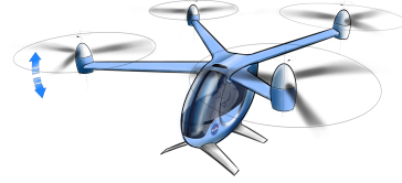
(a) A one-passenger quadrotor design with electric propulsion.
