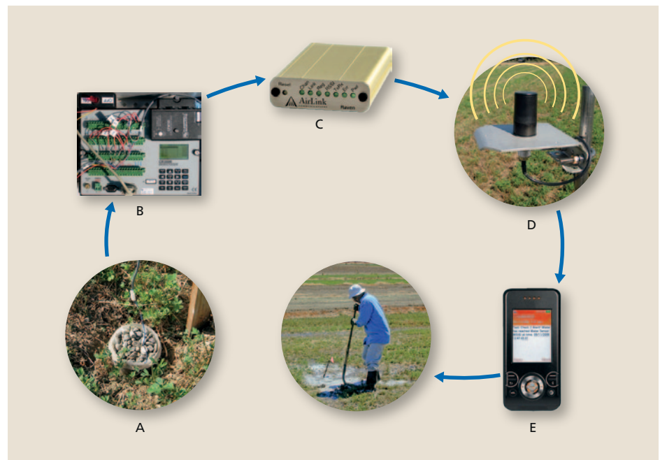
Fig. 2. The cellular communication system contains: (A) wetting-front sensors, (B) central module/data logger, (C) digital cellular modem, (D) cellular antenna and (E) cell phone.
