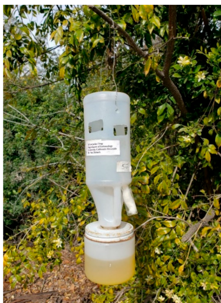
Figure 3. The UCR-style trap with re-useable and interchangeable components.
