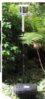
4 microphone sensor node
