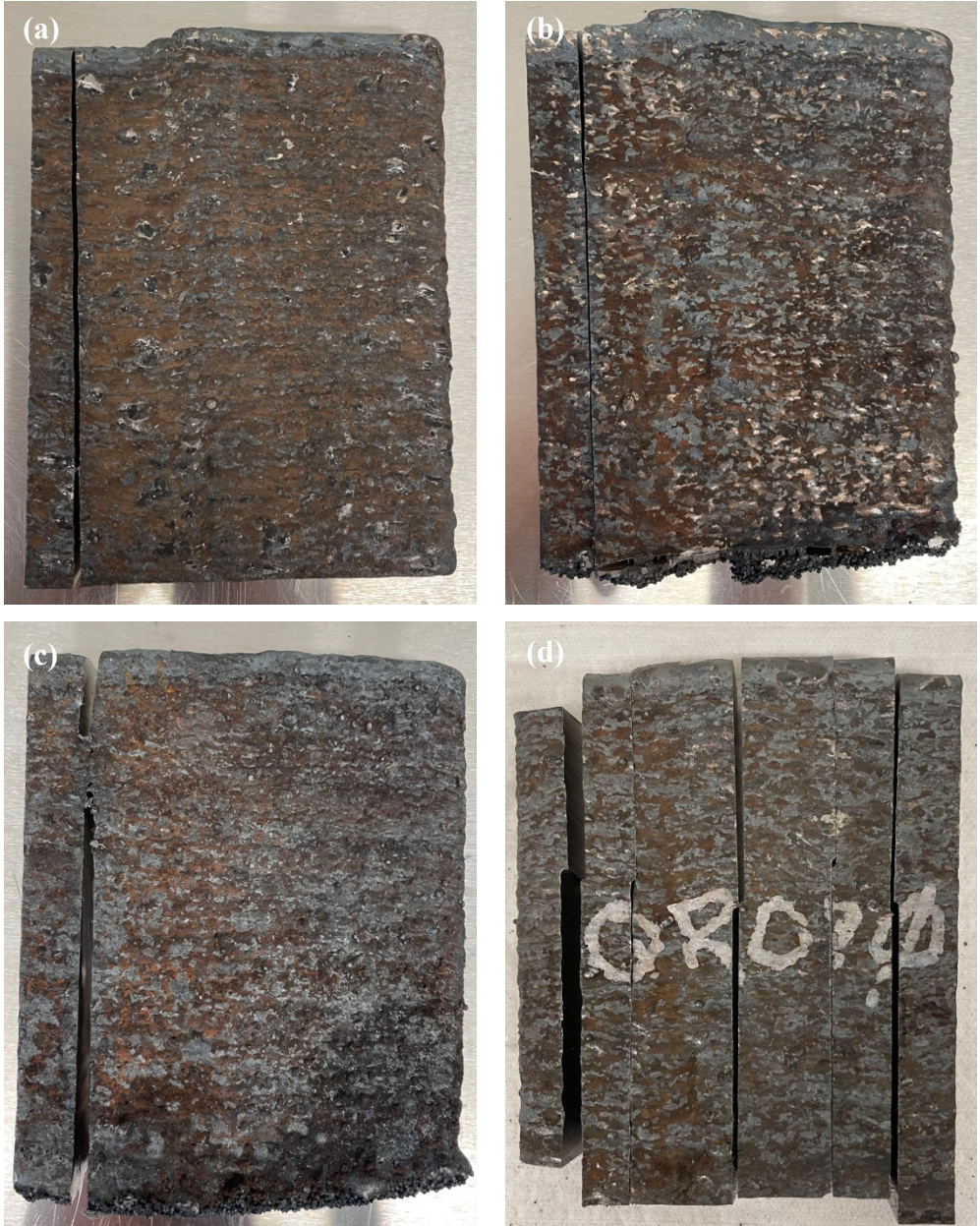
Figure 12: Images of the as-deposited samples for (a) H13 Cored, (b) H13 Solid, (c) Dievar, and (d) QRO 90 produced by Michigan Technological University.
