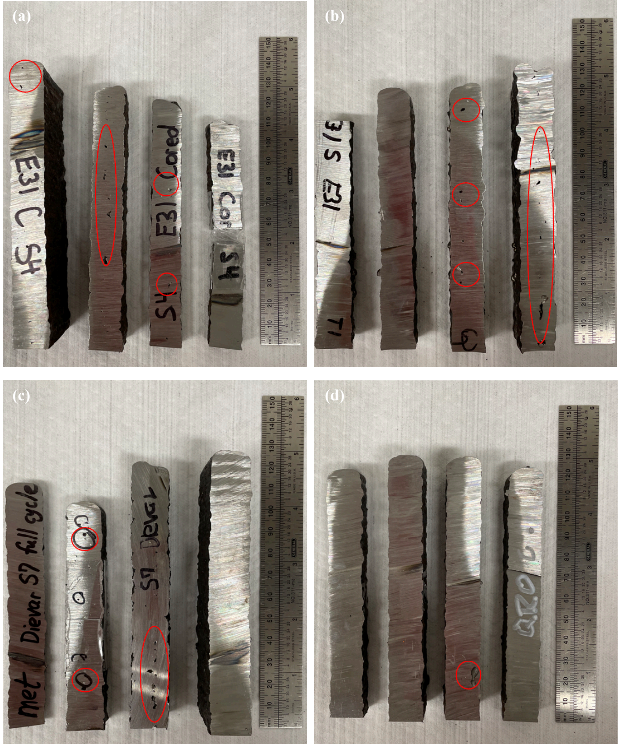
Figure 14: Cross sections of (a) H13 Cored, (b) H13 Solid, (c) Dievar, and (d) QRO 90 with red ovals showing large sized porosity at different locations in the builds.
