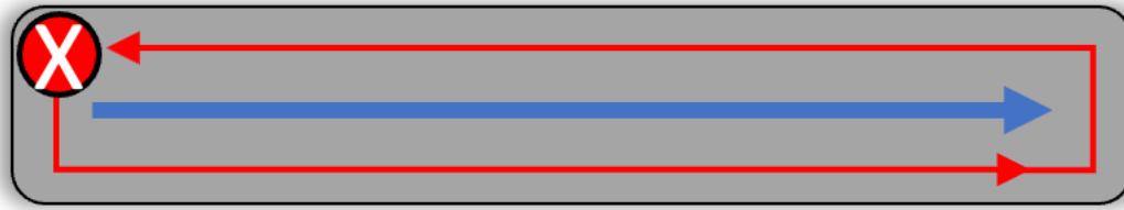
Figure 11: Deposition path used to print the as-built samples. The X denotes the starting point for each layer. The red arrow represents the initial straight bead and the blue arrows represent the subsequent deposition along the perimeter of the first deposition.
