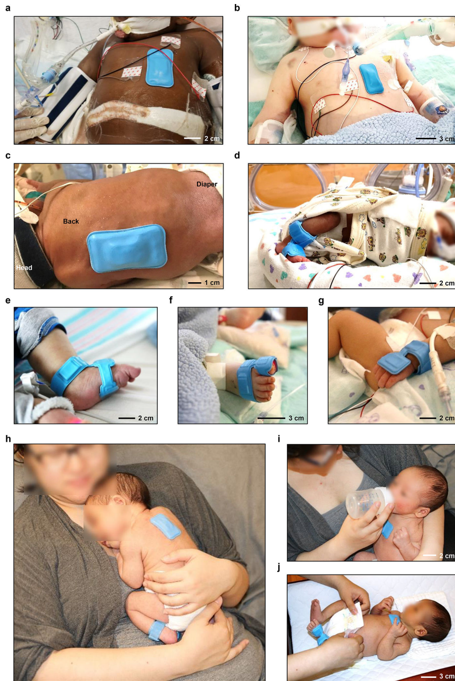
Fig. 3. Photographs of wireless wearable devices on neonatal and pediatric patients in the NICU and PICU, respectively, and of parental hands-on care with healthy neonates. a-c, Photographs of the chest unit on two different ~2-year-old children (a) and (b) and on a neonatal preterm infant in (c) (27 w GA, 6 w CA) with apnea of prematurity and respiratory failure. Here, the device rests on the back. d, Photograph of the limb unit mounted on the ankle-to-foot interface of an infant (27 w GA, 6 w CA) and e, another infant (25 w GA, 44 w CA). f, Photograph of a similar unit on the foot-to-toe interface of the pediatric patient in (b). g, Photograph of a device on the wrist-to-hand interface of a pediatric patient (35 w GA,
