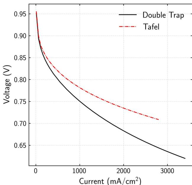
**Figure 4.** Comparison of cathode polarization curves with DT and Tafel kinetics and pure O<sub>2</sub> feed.
