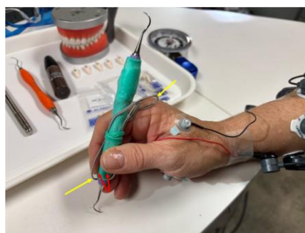
Figure 2: Tester holding test instrument with ultrathin, flexible force sensors affixed to thumb and forefinger grip zones using a thin green sheath. Sensors are not visible, but their location underneath the green sheath is indicated by red arrows. The sensors are connected by fine wires (yellow arrows) to the microcontroller. Some surface Electromyography (sEMG) electrodes and leads are visible.
