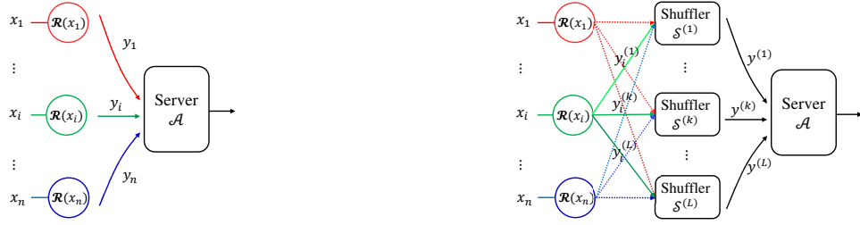
Figure 3.1: DME under privacy and communication constraints: (a) Local differential privacy (LDP) model of n clients. (b) An L -message shuffled (MMS) model of n clients
