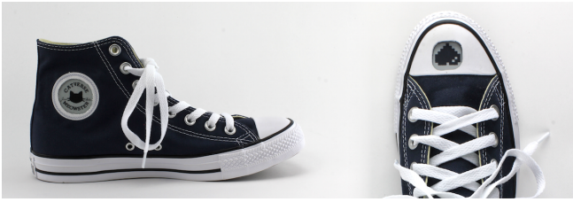
Figure 7. Sneaker prototype. Left: Discreet display on the inside heel of the left shoe. Right: Public display on the toe of the right shoe. AlterWear devices are highly contextual. A single artifact can be both personal and public depending on the location of the display.
