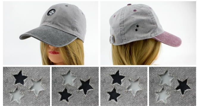
Figure 6. Baseball hat prototypes. Left: Hat prototype with AlterWear display on the front panel. Right: Hat prototype with AlterWear display on the side panel. Below: Close up of the side design. We added a simple animation when updating the display to give the appearance of sparkling or twinkling stars.
