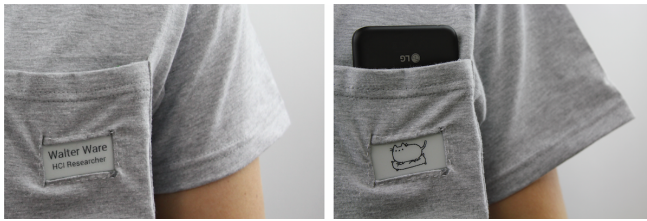
Figure 5. Pocket tee prototype. Left: name tag application. Right: when the user places their NFC-enabled phone in their pocket, the phone continuously powers the display, and a simple animation is displayed.
