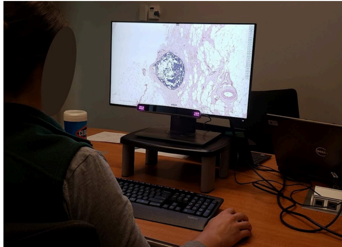
Fig 1. Experimental apparatus. A participating pathologist (face obscured for privacy) interpreting a breast biopsy image during the study, navigating the image by using the computer mouse to click-drag (panning in XY space) and scroll (zooming in Z space). The remote eye tracking device is attached to the bottom of the computer monitor.
