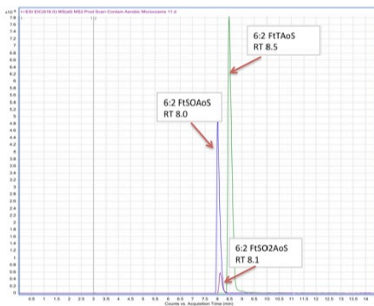
Figure 4.4: Chromatograph of 6:2 FtTAoS (m/z 586), 6:2 FtSOAoS (m/z 602), and 6:2 FtSO 2 AOoS (m/z 618) molecular ions in an aerobic live microcosm on day 29 of incubation.
