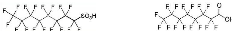
Figure 1.1: Structures of the protonated C_8 perfluoroalkyl acids: (left) perfluorooctane sulfonic acid (PFOS) and (right) perfluorooctanoic acid (PFOA).
