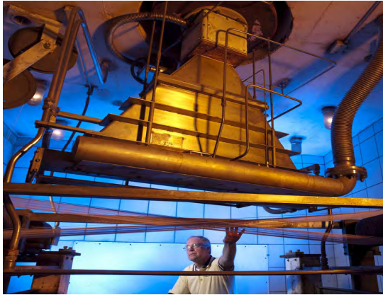
Figure 11: Electron beam cross-linking of polymers improves heat resistance of coatings for wires and cables.
