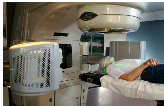
Figure 7: The Varian Medical System for treating a patient with x-ray produced by a high-energy electron beam.
