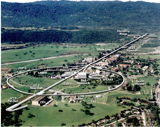
Figure 5: The SLAC site showing the LCLS, a 1.5 Angstrom Free Electron Laser (FEL).
