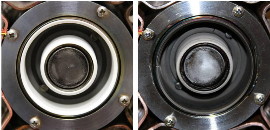
Figure 6.1-2. Comparison of the MaSMi-40's discharge channel before and after approximately 4 hours of operation.
