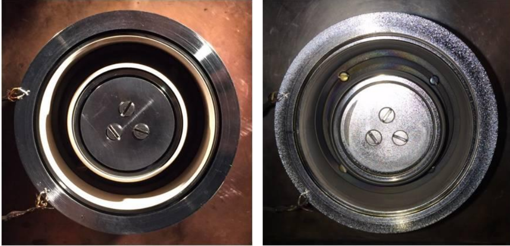
Figure 7.2-4. Comparison of the MaSMi-60's discharge channel and pole faces before and after ~20 hours of operation. Note the level of front inner and outer pole face erosion.
