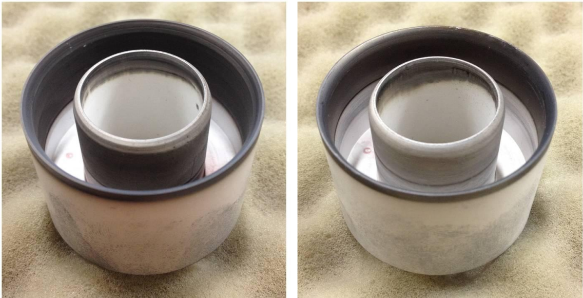
Figure 6.3-1. Comparison of the MaSMi-40's discharge channel after operation in the jet mode (left) and the diffuse mode (right), showing a significant reduction in carbon deposition along the inner wall.
