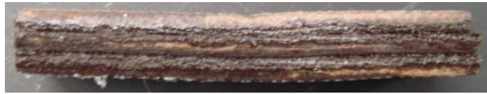
Figure 12: Side view of short beam shear test specimen.
