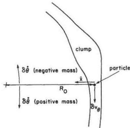
FIG. 2. Negative mass instability. A particle will have a perturbed velocity away from the clump. Because of the geometry, this could cause a perturbed  $\delta\theta$  toward the clump, which would create an instability.
