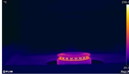
(a) FLIR image of the cooktop burner
