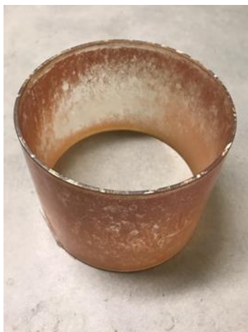
(a) Contaminated quartz tube
