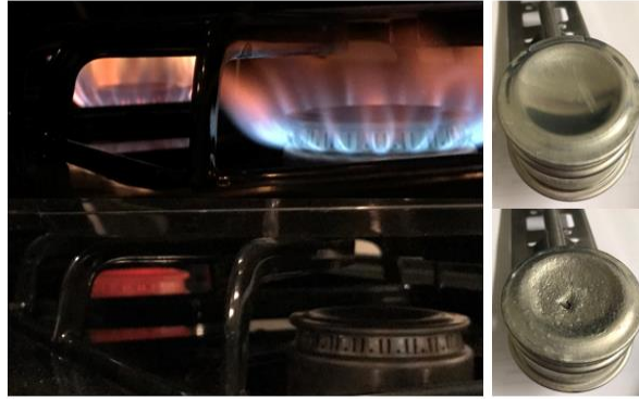
Figure 28: Cooktop burner flashback in the water boiling process
