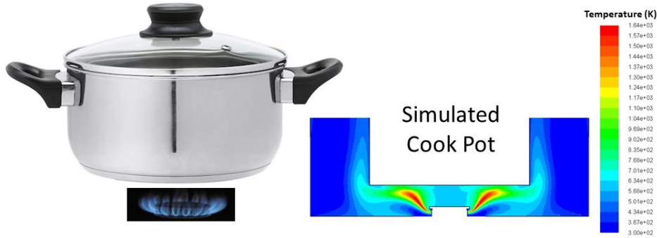
Figure 37: 2-D cooktop burner model
