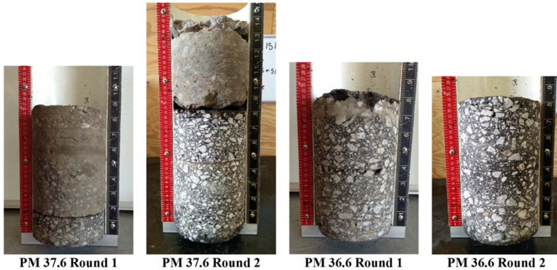
Figure 4.56: Cores from San Luis Obispo 46. (Note: all cores are upside down in the figures.)
