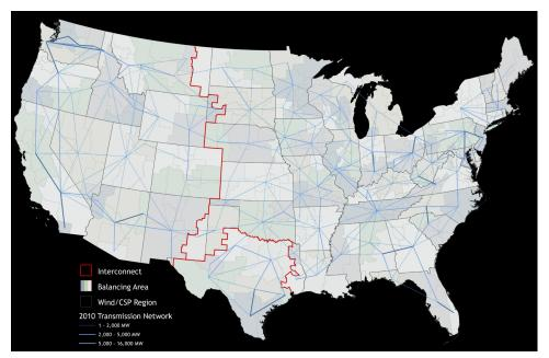
Interconnections are shown here outlined in red. ERCOT, representing most of Texas, is the most isolated region of our study. ERCOT only has three connections outside of its interconnection, while both CAISO and ISO-NE are more connected to neighboring regions and rely on imports for a portion of their generation needs.
