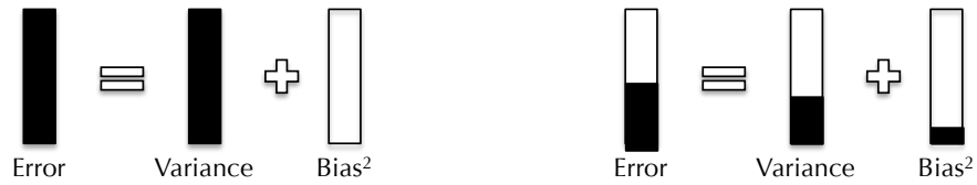
Figure 2.1: (left, traditional MCMC): the error solely comes from the variance error because the samples are unbiased, (right, SG-MCMC): large variance error is reduced by sampling much faster at the expense of allowing some bias error.
