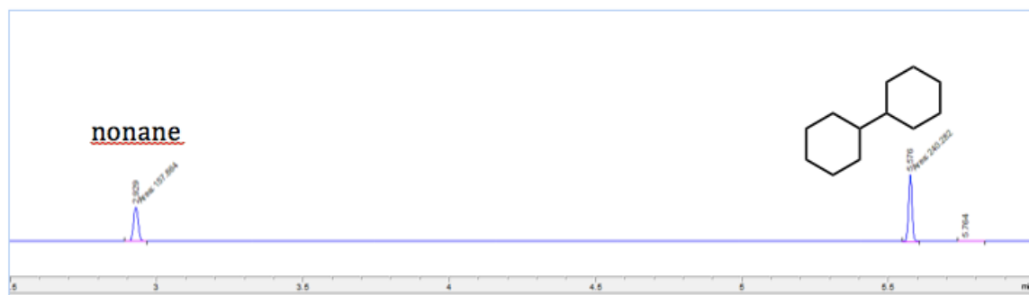
Figure 3.4. GC trace showing one to one mixture of nonane to bicyclohexyl.
