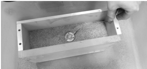
Figure 6. Photo of the load cell placement
