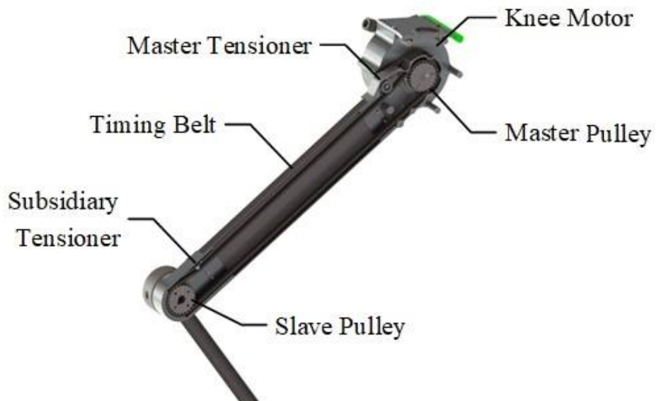
Figure 3.3: Section view of the femur link with the pulley transmission mechanism inside enabling continuous knee rotation.
