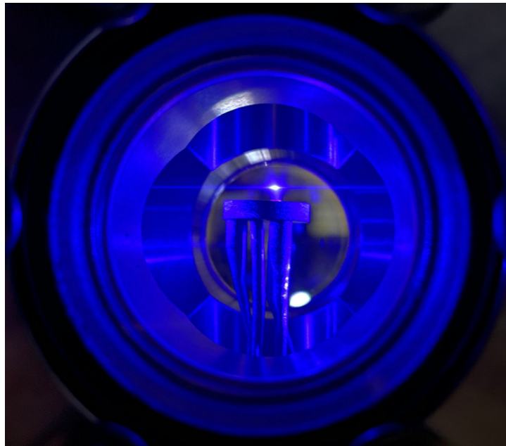
Figure 4.2: 3D-printed titanium oven being tested in a vacuum chamber. Neutral strontium fluorescence at 461 nm can be observed as a brightly glowing dot directly above the oven aperture, and a thin line that traces the path of the laser beam.
