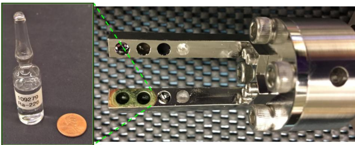
Figure 4.8: 10 \mu\text{g} (10 \mu\text{Ci} ) are contained in a solution of hydrochloric acid (left). This solution is dried into a target holder (right) that is attached to a heavy duty linear push-pull feedthrough.
