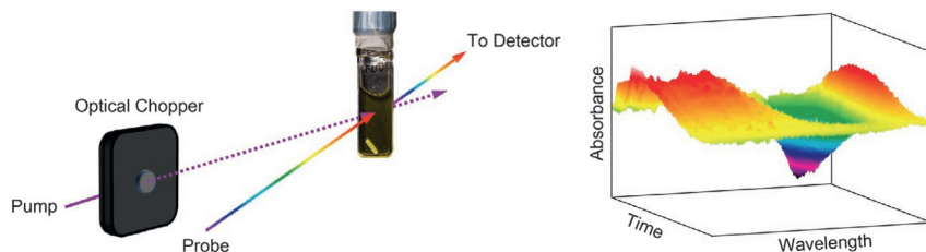
Fig. 4 Schematic of the light pulses utilized in an ultrafast transient absorption experiment ( left ) and a representative plot of the resulting data ( right ). Photochemistry is initiated in the sample by the pump beam which has previously been passed through an optical chopper to remove every other pulse. Changes in the sample are measured by the probe beam which is composed of a white light continuum of wavelengths from \sim 350 – 800 nm (when using \text{CaF}_2 crystal). It is directed onto the sample at the same position as the pump beam and then passes to a detector, while the pump is blocked. A light-minus-dark absorption spectrum is generated for all wavelengths and a three-dimensional plot is constructed displaying the kinetics at each wavelength in one direction (i.e., the yz plane) and full absorption spectra for each time point in the other direction (i.e., the xy plane).
