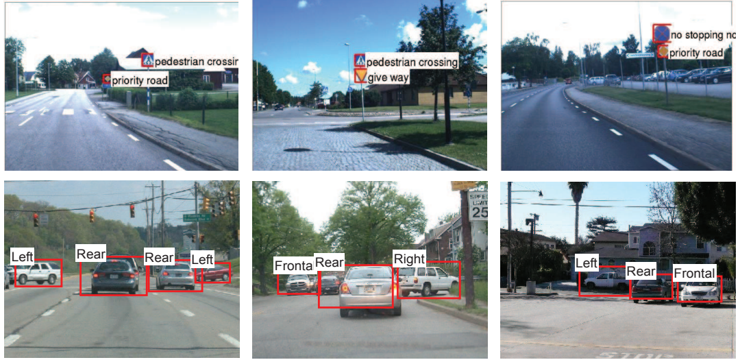
Figure V.6: Examples of detections of cars from different views and several traffic signs.
