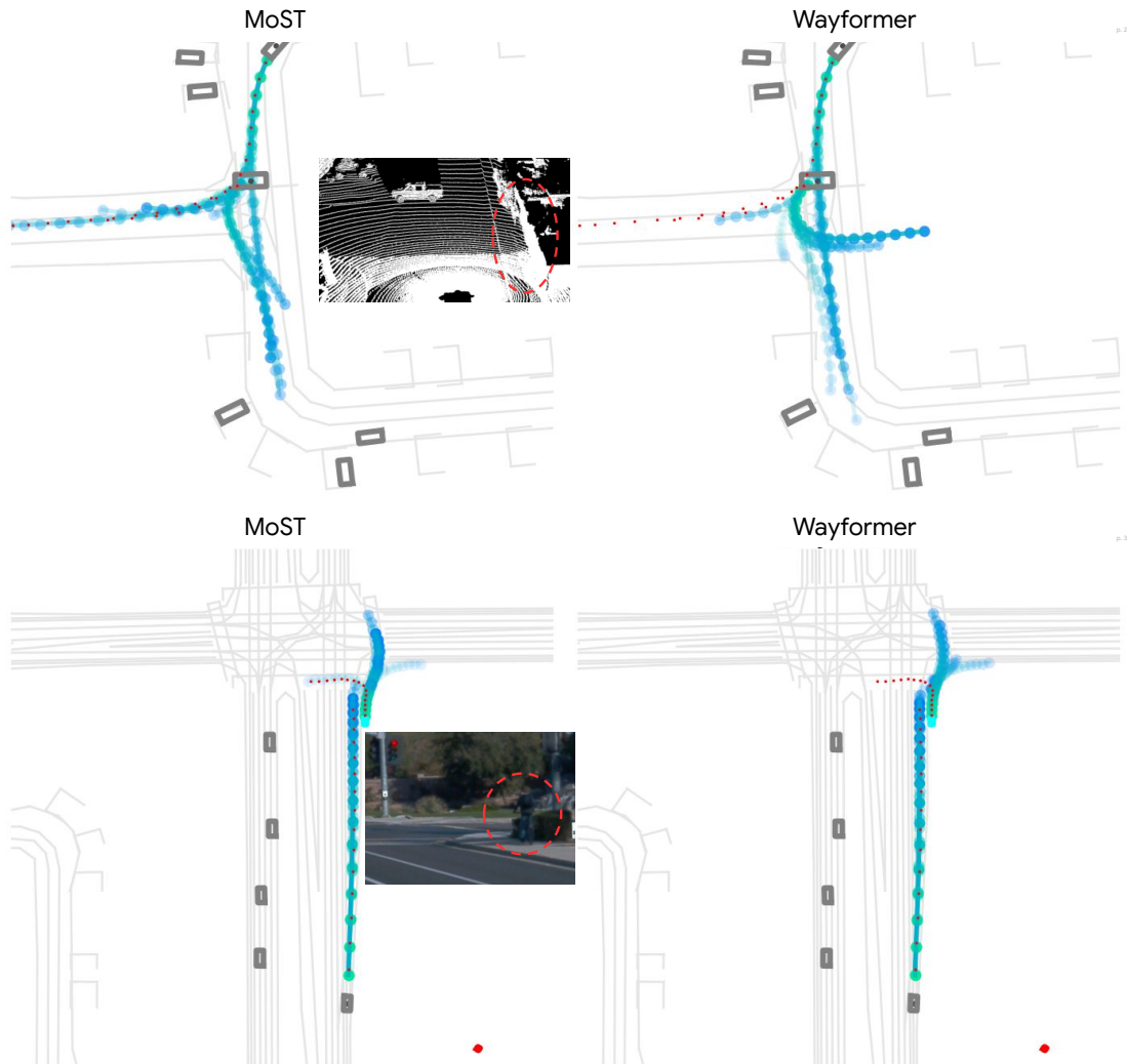
Figure 3.5: Qualitative comparison. The agent boxes are colored by their types: gray for vehicle, red for pedestrian, and cyan for cyclist. The predicted trajectories are ordered temporally from green to blue. For each modeled agent, the models predict 6 trajectory candidates, whose confidence scores are illustrated by transparency: the more confident, the more visible. Ground truth trajectory is shown as red dots. In the upper example, MoST rules out the possibility that a vehicle runs onto a wall after U-turn; in the lower example, MoST correctly predicts that a cyclist could suddenly cross the street.
