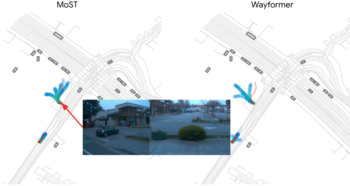
Figure 3.6: Additional qualitative comparison between MoST and Wayformer (Nayakanti et al., 2023) baseline. The agent boxes are colored by their types: gray for vehicle, red for pedestrian, and cyan for cyclist. The predicted trajectories are ordered temporally from green (+0s) to blue (+8.0s). For each modeled agent, the models predict 6 trajectory candidates, whose confidence scores are illustrated by transparency: the more confident, the more visible. Ground truth trajectory is shown as red dots. Note that the vehicle indicated by the red arrow is entering a plaza which has no map coverage. Since our model has access to the rich visual signals, it correctly predicts the vehicle’s possible trajectory which includes follows the arrow and turn right. Wayformer, on the other hand, completely missed this possibility due to the lack of road graph information in that region.
