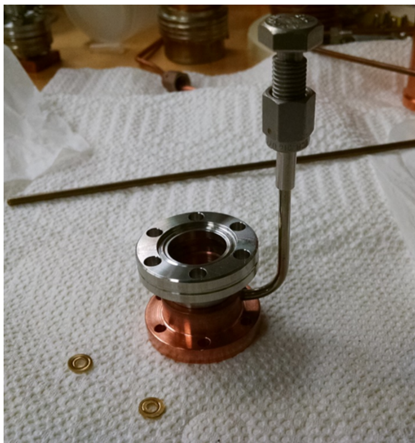
Figure 3.6: A picture of the helium-4 evaporative refrigerator pot. The capillary tube impedance is housed in a VCR fitting that is attached to the small protruding pipe. The top of the pot connects directly to a larger diameter CF pipe to efficiently evacuate evaporated helium gas.
