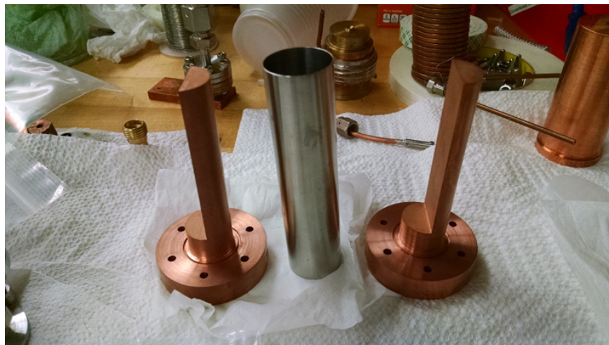
Figure 3.9: The heat switch before brazing assembly.
