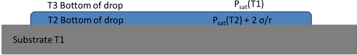
Figure 3.19: Simple heat transfer model for a drop on the sapphire substrate, not to scale.
