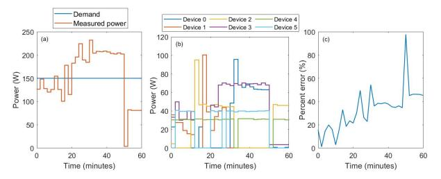
Figure 4.2. Scenario 1 for the system without a battery. Timeseries of a) individual device power, b) reference signal and measured total power, and c) percent error with respect to demand signal.
