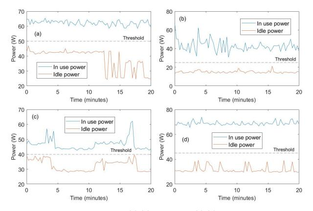
**Figure 3.1.** Power profiles for (a)-(b) laptops and (c)-(d) tower computers with threshold used to determine the mode of operation (in use versus idle) of the loads
