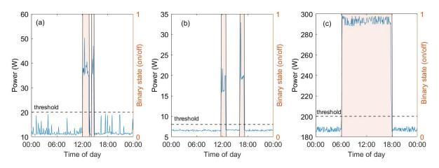
Figure 2.1. Daily energy consumption profile measured at 5 min intervals for: (a) Computer, (b) Printer, (c) TV. Red background represents the On state of the loads if the control scheme discussed in this section is implemented
