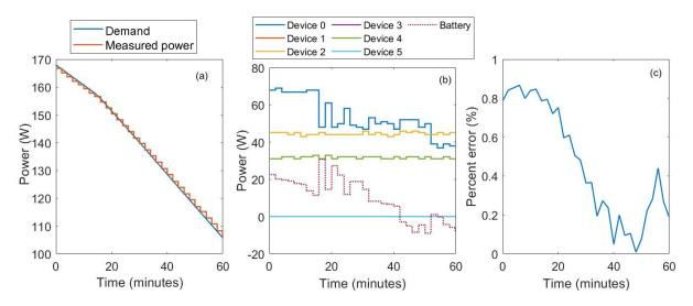
Figure 4.5. Scenario 2 for the system with a battery. Timeseries of a) individual device power, b) reference signal and measured total power, and c) percent error with respect to demand signal.
