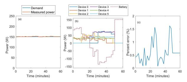
Figure 4.3. Scenario 1 for the system with a battery. Timeseries of a) individual device power, b) reference signal and measured total power, and c) percent error with respect to demand signal.
