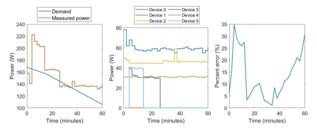
**Figure 4.4.** Scenario 2 for the system without a battery. Timeseries of a) individual device power, b) reference signal and measured total power, and c) percent error with respect to demand signal.
