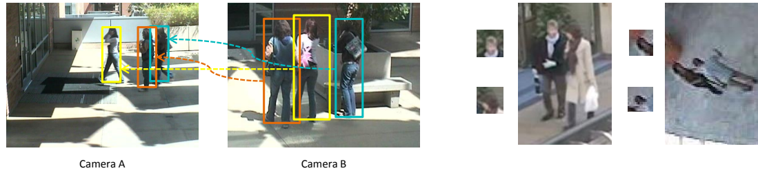
Figure 1.6: (Left) Social grouping behavior not only generally exists in one scene, but also usually persists (with the same group members) across wide areas. (Right) Given head images alone, it is sometimes difficult for human beings to correctly identify head pose directions in challenging scenarios. Social context provides strong evidence for this difficult problem.
