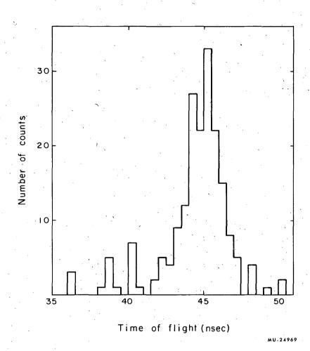
Fig. 8(C). Time-of-flight histogram of K mesons at 900 Mev/c, using Cerenkov counter C1 to produce the trigger.
