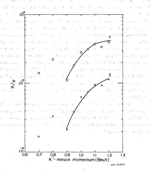
Fig. 11. Production of K mesons at different momenta. Curve E gives actually counted  $K/\pi$  ratios during the run. Curve T is the  $K/\pi$  ratio at the Bevatron internal target, obtained by correcting the actual counts for decay in flight.
