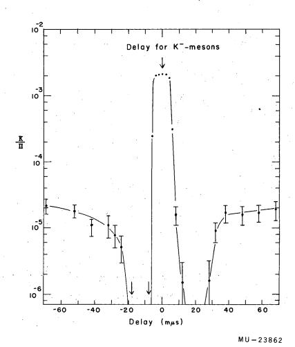
Fig. 7. Delay curve obtained by delaying B<sub>3</sub> and B<sub>4</sub> in the main K-selecting coincidence circuits. This illustrates the effectiveness of the anticoincidence signals from the Cerenkov counter.
