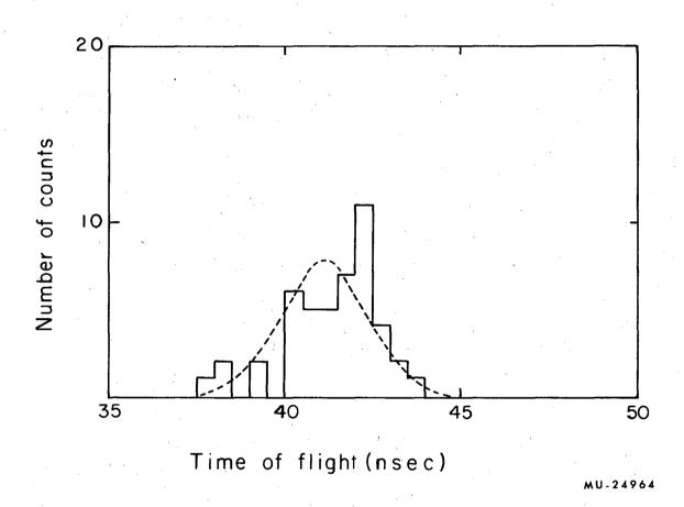
Fig. 8(B). Time-of-flight histogram of π mesons at 900 Mev/c nominal momenta, obtained by triggering the oscilloscope with the coincidence of beam counters B<sub>1</sub>, B<sub>2</sub>, B<sub>3</sub>, and B<sub>4</sub>.
