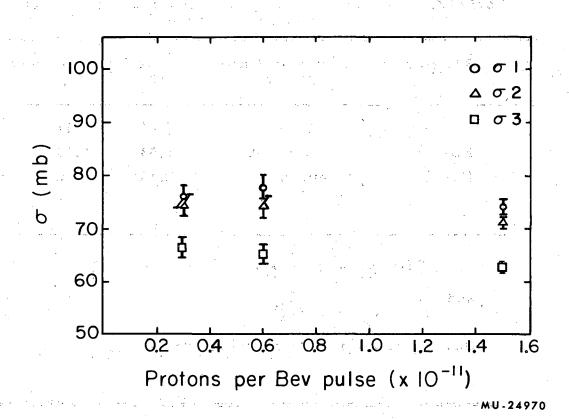
Fig. 13. Measured K -D cross section vs proton beam intensity at 1150 Mev/c nominal momenta for the three transmission counters. Within statistical errors the cross sections do not depend on beam level.
