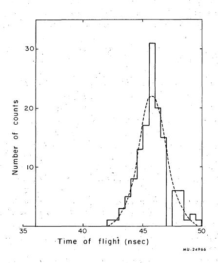
Fig. 8(A). Time-of-flight histogram of K mesons at 900 Mev/c nominal momenta, obtained by triggering the oscilloscope with the K signal.
