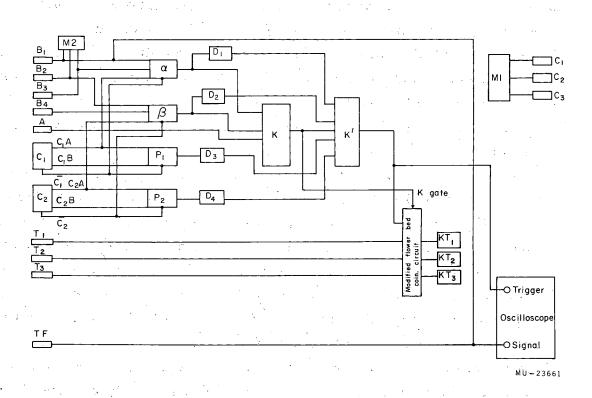
Fig. 5. A simplified schematic drawing showing major electronic components: a, β, P<sub>1</sub>, P<sub>2</sub>, and K are fast coincidence-anticoincidence circuits; D<sub>1</sub>, D<sub>2</sub>, D<sub>3</sub>, D<sub>4</sub> are delay boxes. K' is a Garwin coincidence circuit. The modified flower bed circuit is a multichannel double-coincidence circuit.
