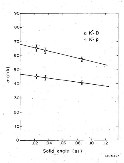
Fig. 12. Solid angle subtended by the transmission counters vs measured uncorrected total cross sections (only accidental corrections included) at 900 Mev/c nominal momenta. Note the linear dependence of both K -p and K -d total cross sections.
