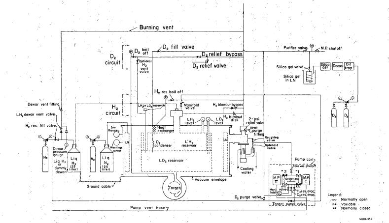
Fig. 3(B). Schematic drawing of the whole hydrogen-deuterium target system.
