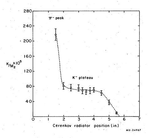
Fig. 6. Cerenkov radiator position-plateauing curve. The K mesons were counted by fixing the radiator position at the center of the approx 3-in. -wide K meson plateau.
