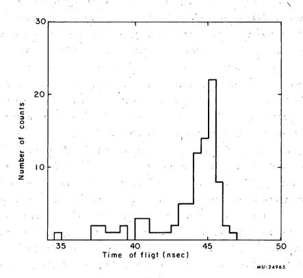
Fig. 8(D). Time-of-flight histogram of K mesons at 900 Mev/c, using Cerenkov counter C2 to produce the trigger.
