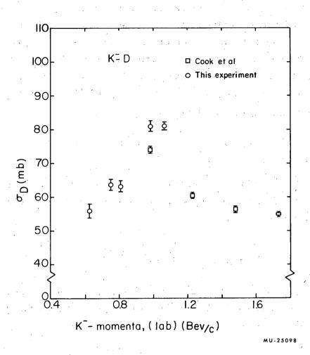
Fig. 16. The K-d total cross sections plotted together with some of the data from the experiment of Cook et al. We measured the K-d cross sections at fewer points and with less statistical accuracy.
