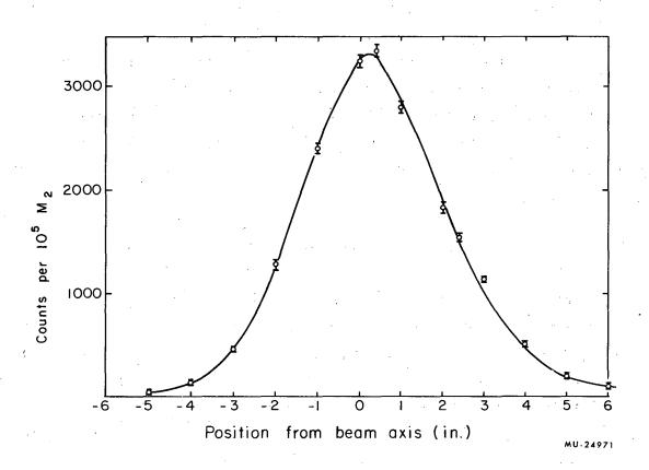
Fig. 14. Horizontal beam profile obtained by using a 1/2-in.-sq scintillation counter. The vertical profile is very similar to the horizontal.
