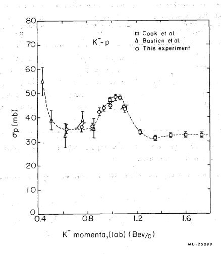
Fig. 15. The K -p total cross sections plotted together with some of the data from the experiment of Cook et al., 5 and some preliminary data of Bastien et al. 6 (I would like to thank Professor Robert D. Tripp for communicating the unpublished data from his group). The resonant peak appears about 15 mb above the nonresonant background of approx 35 mb (see also Table X).
