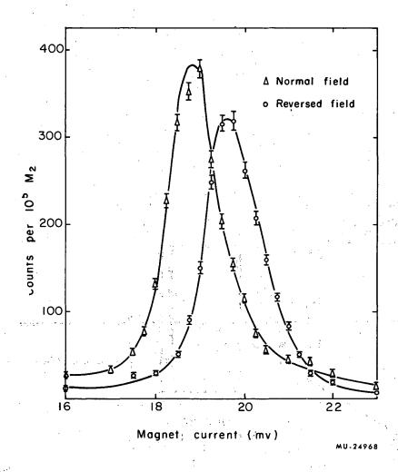
Fig. 10. Typical curves obtained during momentum measurement of the beam particles. One curve is for one sign of the magnetic field, the other is for the reversed field. An average of the two gives the actual momentum of the beam particles passing through the analyzer magnet.
