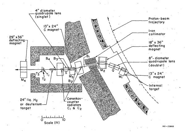
Fig. 2. Arrangement of K beam. M, M2, and M3 are bending magnets, Q is a quadrupole doublet and S is a quadrupole singlet lens. Scintillation counters B1, B2, B3, and B4 define the beam, and T1, T2, and T3 measure the transmission.
