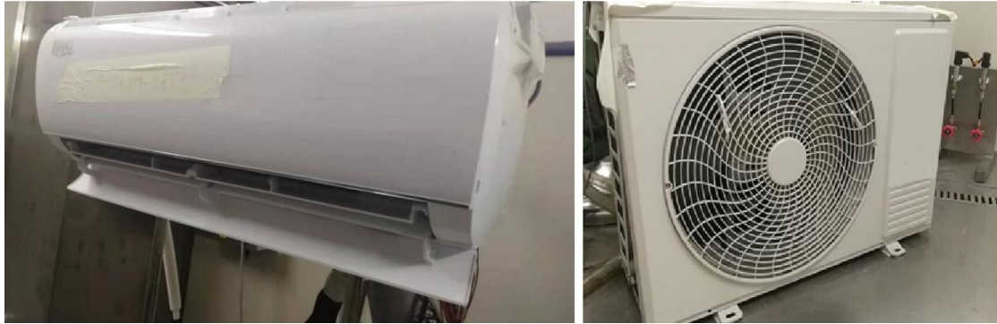
Fig. 3. Photographs of the R32 prototype AC unit.
