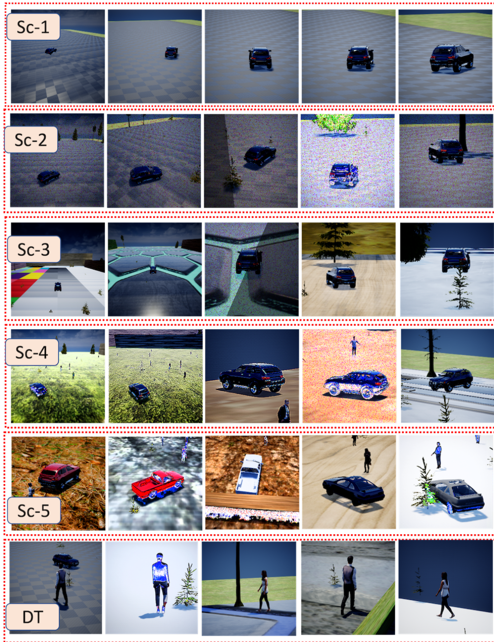
Figure 5.5: Visualization of scenarios shown in Table 5.2. Sc-1 has a fixed background. In Sc-2, fixed background is extended with random tree placements and image augmentations. Sc-3 shows background variations with image augmentations and trees. Sc-4 extends the Sc-3 scenes with humans and same vehicle with different colors. In, Sc-5, we add vehicles of different types as well. DT shows the scenes for dynamic tasking of policy to track human characters.
