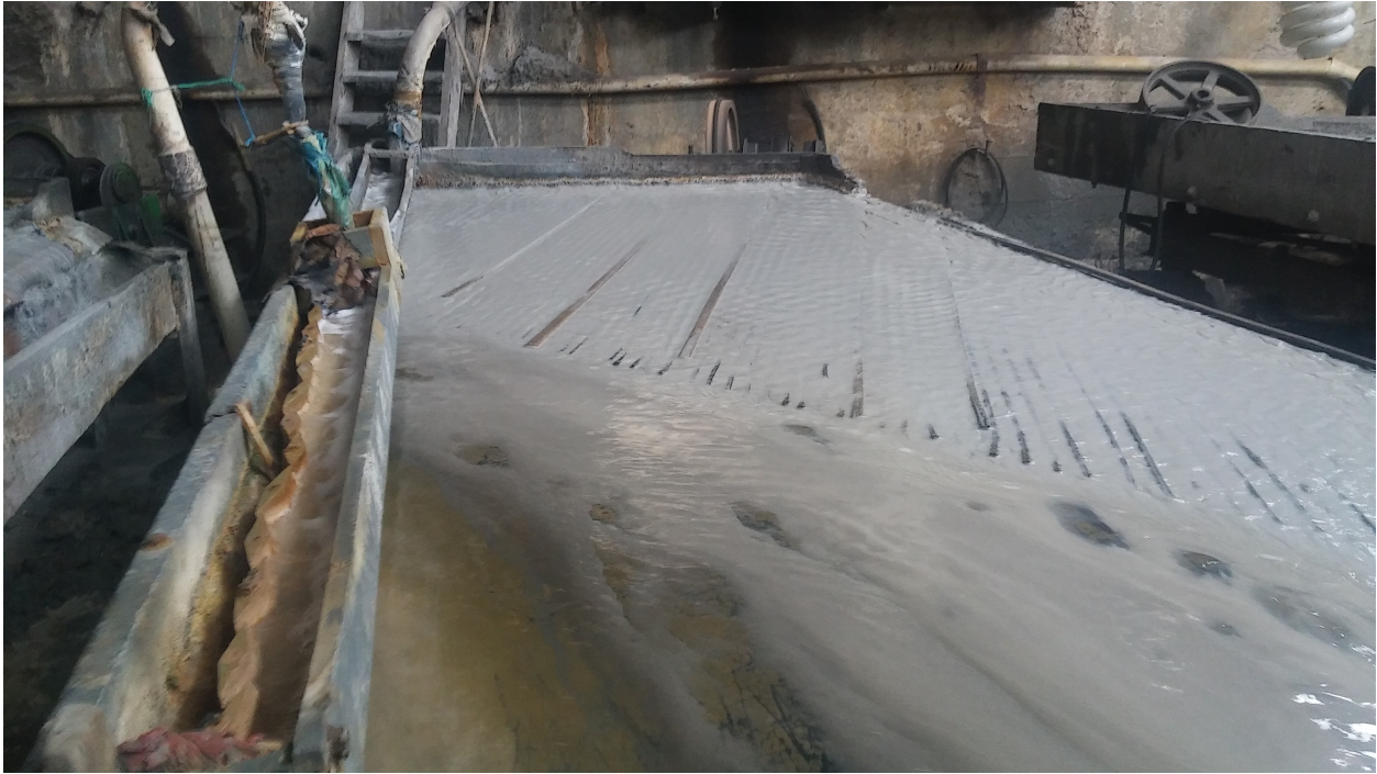
Figure 23: Shaking Tables and Metallic Streaks, Sink & Float Plant. February 9, 2017.
