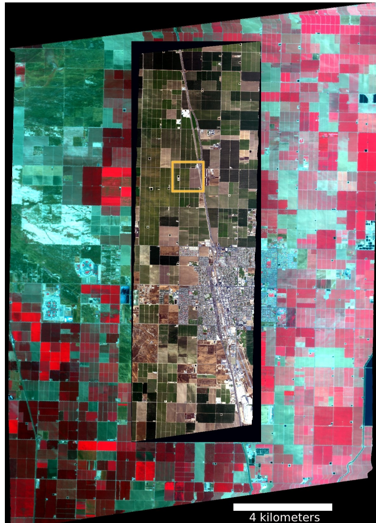
Figure 2.7: MASTER and AVIRIS flightlines; yellow box is the field site shown in Figure 1. MASTER bands: Red = 9, Green = 5, Blue = 3 ; AVIRIS bands: Red = 29, Green = 20, Blue = 11
