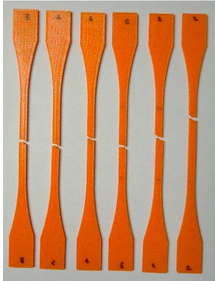
Figure 3.13: Failed samples of modified geometry. Note that they all broke within the 25 mm gauge region.
