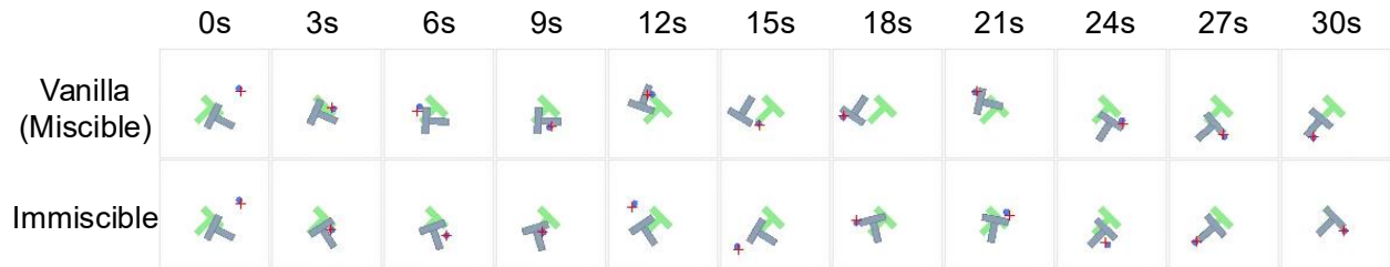
Figure 5.7: Immiscible diffusion boosts the performance of diffusion policy. Here the robot (circle) needs to push the T-shaped object (gray) into the desired place (green).
