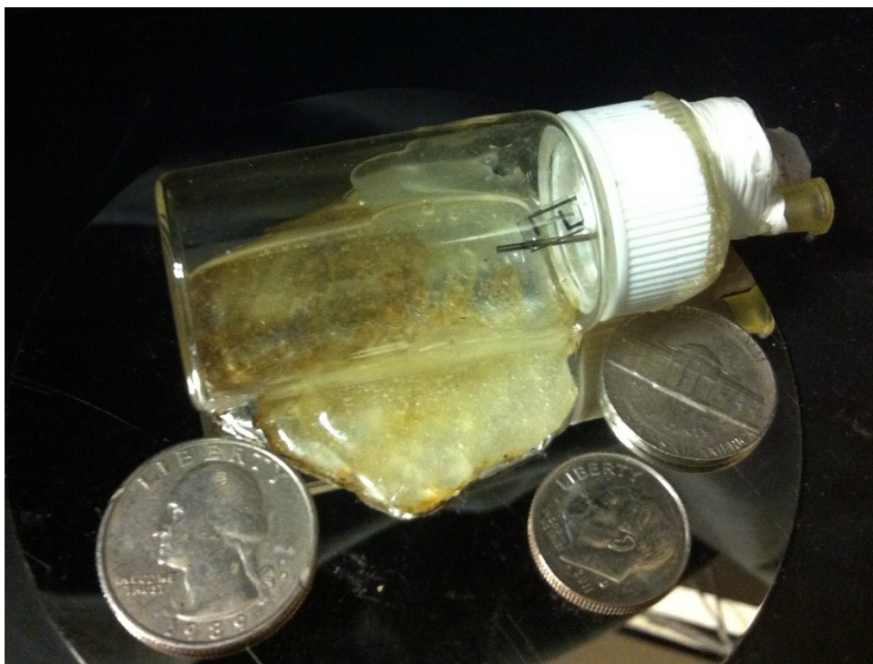
Figure 3.1: Picture of IDA electrode set-up, with coins shown for scale. Needle inlets, two, are located below the IDA electrode which faces up. One needle is large enough to allow for a smaller needle to be threaded through it to add the microliters of solvent.
