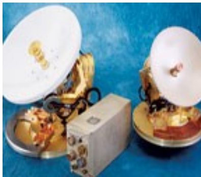
Fig. 1-4. 45 & 30 cm diameter Ka-band aeronautical mobile satcom tracking reflector antenna systems. (Photo from www.L-3com.com Datron division)
