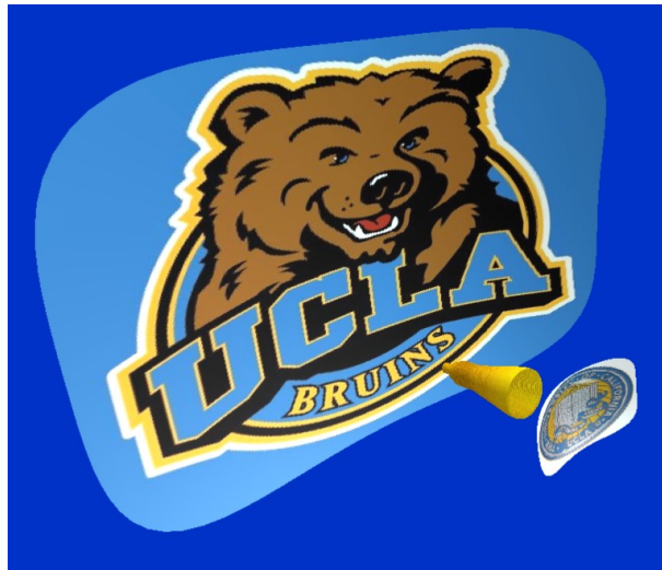
Fig. 8-7. Example display of DUAL reflector geometry with super quadratic main and subreflector apertures, (peculiarly stubby Cassegrain system for example only) along with the feedhorn. 3D graphics produced by the ARAM CYL_MM Windows™ software developed for this dissertation.
