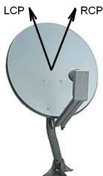
Fig. 7-1. Squinted (exaggerated) CP beams from an offset reflector. (Photo from www.ebay.com )
